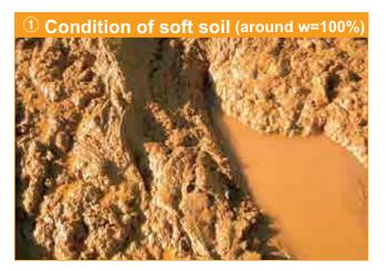
Niigata Chuetsu earthquake caused large volume of soft soil. But it was improved in-situ, and activating surface compaction. It means that this contributed to prompt disaster recovery.
