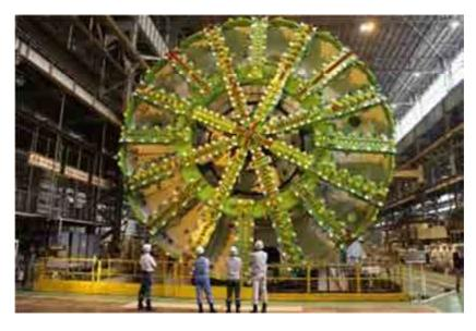
**Photo.1** Shielded machine with a diameter of about 16 m
