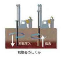
Figure 2 Structure of pile removal
