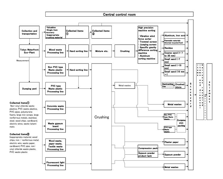
Figure 1 System flow of "High precision sorted recycling system"
