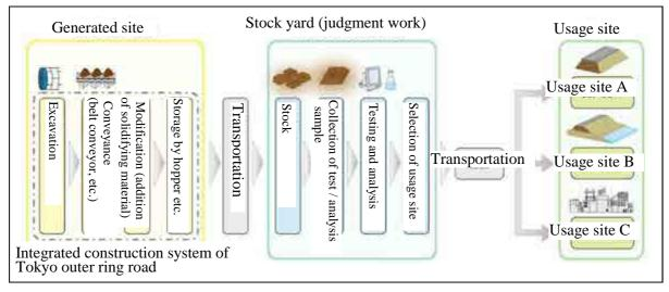
Fig. 3 Flow of management of shield generated soil
