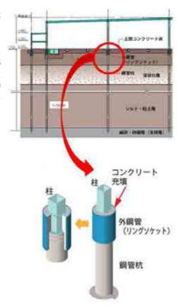
Figure 3 Sectional view of building and pile head ring socket
